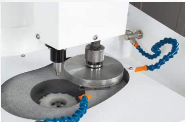
Prepolishing of large raw samples.
