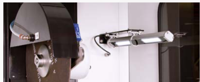
Work area lit by LED strip
