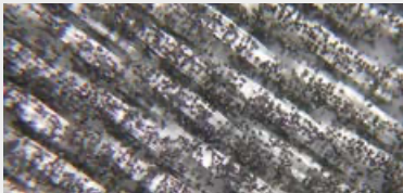
Polycrystalline diamond on cloth
